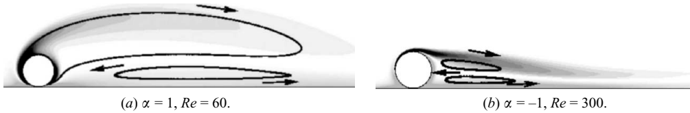
FIGURE 6. Vorticity contours for the steady flow around the cylinder. The streamlines showing the presence of the two recirculation zones are overlaid in black. The streamlines are shown in the frame of reference attached to the cylinder centre.
